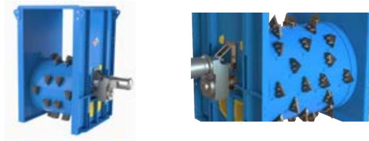
Breaks and fluffs up material. Optional knives can be used to open bags and break up green waste.
