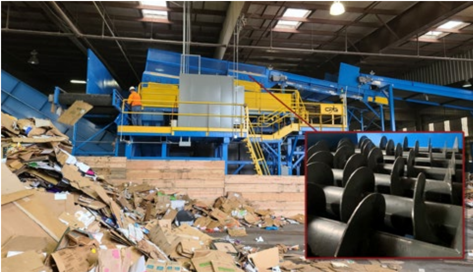
▲ The patented CP Elliptical Auger Screen scalping cardboard from commercial and industrial material recycling streams.
